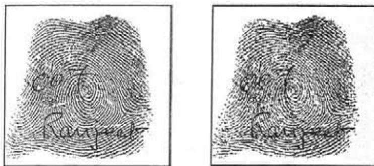
Figure 1.7: Fingerprint image after using sharpen and unsharp mask filter of fingerprint image of Figure 1.3
